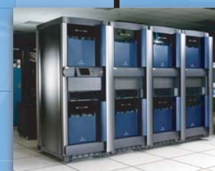
1997 • Turing SGI Origin 2000 • 24 CPUs • 195 MHz Peak Performance: 9.36 GFLOPS
