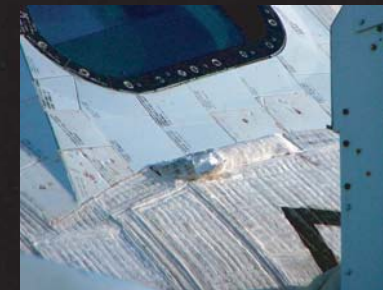
Post-flight photo of the torn 20 x 3 inch panel of the Advanced Flexible Reusable Surface Insulation blanket located under the commander's window on the Discovery Shuttle. (Image courtesy of NASA Orbiter Ops and Project Mgmt Office)
