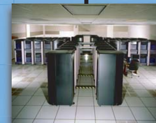
1999 • Lomax SGI Origin 2800 • 512 CPUs • 400 MHz Peak Performance: 409.60 GFLOPS
