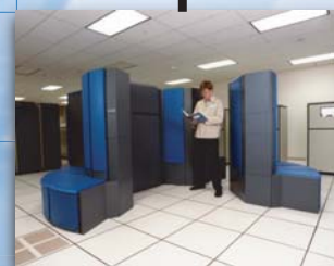
1988 • Reynolds Cray Y-MP • 8 CPUs Peak Performance: 2.54 GFLOPS
