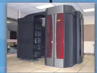
2004 Cray X1 • 16 CPUs • 800 MHz Peak Performance: 51.20 GFLOPS
