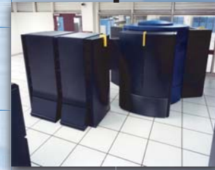
1993 • von Neumann Cray C90 • 16 CPUs Peak Performance: 15.36 GFLOPS
