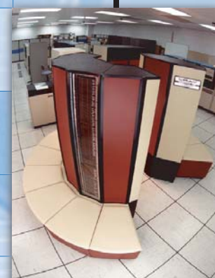
1985 Cray X-MP 12 • 1 CPUs Peak Performance: 0.21 GFLOPS
