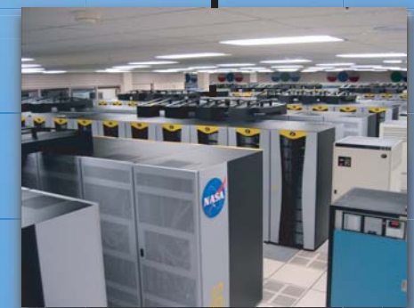
2004 • Columbia SGI Altix 3700 • 10,240 CPUs • 1.5 GHz Peak Performance: 61.44 TFLOPS
