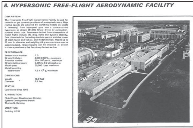
N-237, Diagram of Hypersonic Free-Flight Aerodynamic Facility, 1974 (Source: NASA Ames Facilities Summary, 1974)
