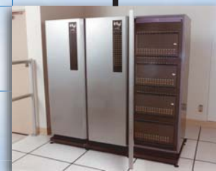
1990 • LaGrange Intel iPSC/860 • 128 CPUs Peak Performance: 7.68 GFLOPS
