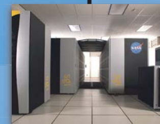
2003 • Kalpana SGI Altix 3000 • 512 CPUs • 1.3GHz Peak Performance: 2.66 TFLOPS
