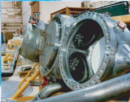
Pictured here is the redesigned two-duct hot gas manifold hardware (new powerhead design), which is considered the backbone of the Shuttle engine, and consists of the main injector and two preburners, or small combustion chambers, in addition to various propellant and oxidizer pumps, ducts, and lines. (Photo courtesy of Rocketdyne)
