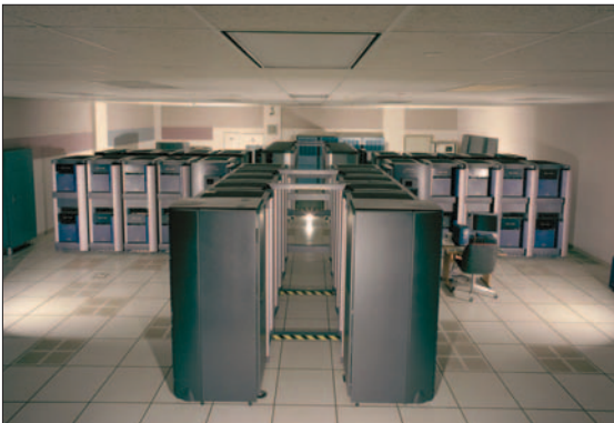
N-258, NAS Origin 2000 Computer System - 512 Processor ("LOMAX") station, 30 September 1999 (Source: NASA Ames Research Center, AC99-0195-2)
