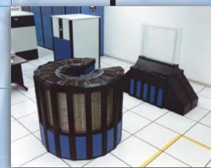
1985 • Navier – 1987 • Stokes (pictured) Cray 2 • 4 CPUs Peak Performance: 1.95 GFLOPS
