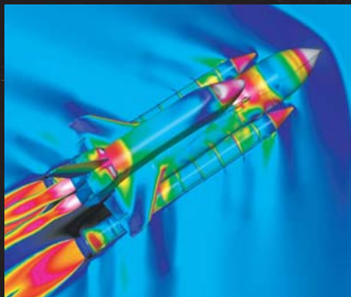
This image illustrates the OVERFLOW solution of the Space Shuttle Launch Vehicle flowfield at a Mach number of 1.25. The vehicle surface is color-coded by the pressure coefficient, and the color contours in the flowfield and plumes represent the local Mach number. (Image generated by Reynaldo Gomez, NASA Johnson Space Center)
