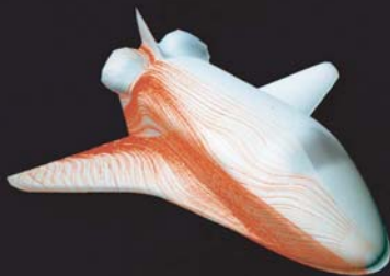
*First ever Navier-Stokes solution of the complete configuration of the Shuttle Orbiter. Calculated at Mach 1.4 and zero degree angle of attack. (Image generated by G. Bancroft and F. Merritt, Applied Computational Fluids Branch, NASA Ames Research Center)
