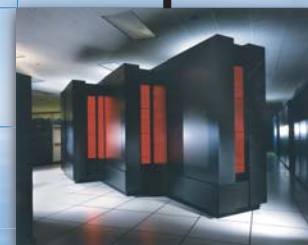
1993 • Boltzmann Thinking Machines CM5 • 128 CPUs Peak Performance: 16.38 GFLOPS
