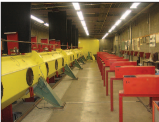
N-237, interior of Hypervelocity Free Flight Facility, test chamber (left) and cameras (right) (Source: Page & Turnbull)
