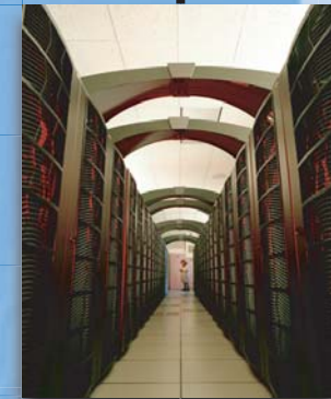
2001 • Chapman SGI Origin 3800 • 1,024 CPUs • 600 MHz Peak Performance: 1.23 TFLOPS
