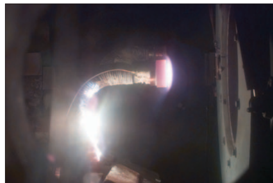
N-238, Reinforced Carbon-Carbon (RCC) Johnson Space Center model testing in Ames Interaction Heating Facility IHF-127 (Source: NASA Ames Research Center, ACD02-0036-017)
