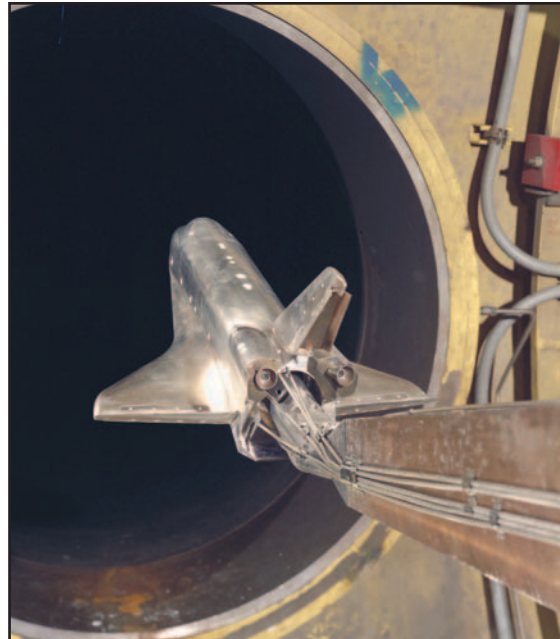
N-229, Space Shuttle Orbiter Model 140A/B-0A87 testing in 3.5-Foot Hypersonic Wind Tunnel, 19 October 1973 (Source: NASA Ames Research Center, AC73-5027)
