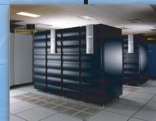
1996 • Newton Cray J90 • 36 CPUs Peak Performance: 7.20 GFLOPS
