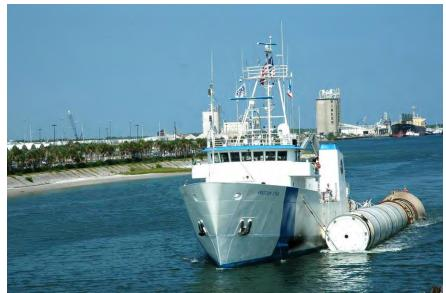
**Photo 3.9.** Retrieval ship *Freedom Star* towing SRB. (Source: NASA John F. Kennedy Space Center, 05PD-1788)
