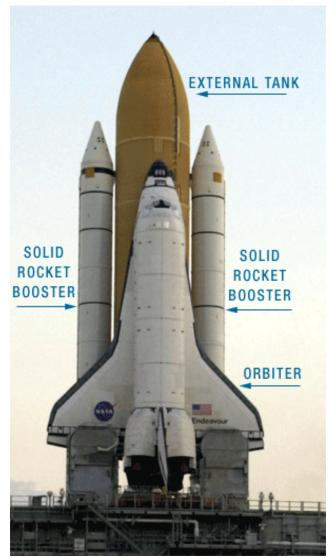
Photo 3.1. The Space Shuttle system. (Source: NASA)
